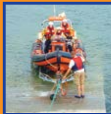
Fully equipped 6.8m RIB with twin 90hp engines and qualified voluntary crew.
