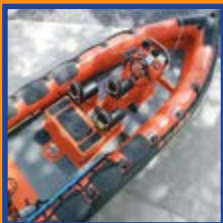
Fully equipped 6.8m RIB with twin 90hp engines and qualified voluntary crew.
